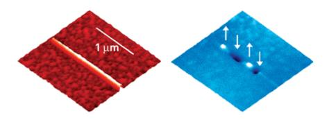
**POLARIZED** Scanning probe micrographs show that small domains in a 12-nm diameter BaTiO<sub>3</sub> nanowire (left) can be manipulated deftly. Using a tip that's biased positively and then negatively, adjacent regions of the wire can be polarized in either orientation (right).
